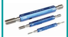
Thread gauging is recommended wherever precision threads are required. The quality of the tapped hole which accommodates the insert determines the finished size and hole quality after the insert has been installed. If the finished tapped hole gauges satisfactorily, the installed insert will be within the thread tolerance. Gauges are available in 2B or 6H or 5H and 3B or 5H or 4H5H
