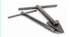
Should inserts need to be removed, the use of the Recoil extraction tool is recommended. Extraction tools are simple and easy to use. As correct positioning will make the extraction easier, the tool should be turned 90° from the start of the coil allowing easy winding out of the insert. If the extraction tool is not gripping the insert, the edges can be re sharpened. Sizes available are M2 to M65 and equivalent Inch sizes.
