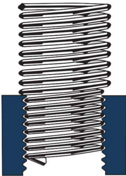
Recoil insert in semi-installed position
